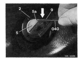
20 On both steering lock versions, insert collar into instrument panel.
