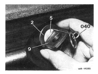
12 Remove cap including locking cylinder from steering lock. Pull releasing wire out of locking cylinder. Turn ignition key to position "0" and pull out.
