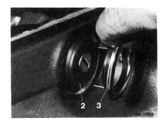
C. Complete removal and installation of steering lock
