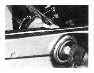
40 On diesel vehicles without steering lock starter switch, attach cable control for preglow starter switch to steering lock, while paying attention to dimension "a", which should amount to  $22.7 \pm 0.5$  mm. If required, set to correct dimension by adjusting knurled screw on pre-glow starter switch. Reference dimension "b" = 165 mm.
