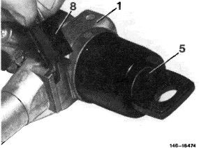
21 With steering lock 2nd version in position "1", push-in detent (6) and remove locking cylinder (5) from steering lock.
