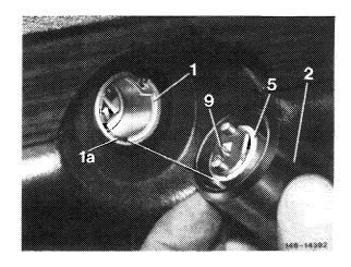
13 Remove locking cylinder from cap.
