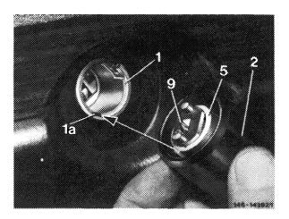
33 Screw cap completely on steering lock.
