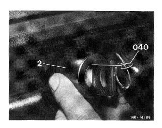
34 Pull releasing wire from locking cylinder. Turn cap to the left (max. 1 turn) until detent of locking cylinder engages in groove of cap.
