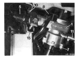
19 Push-in locking pin (10) for steering lock (6) with a punch approx. 3 mm thick (refer to arrow). Slightly turn steering lock. Turn ignition key into position "0" and pull out. Remove steering lock from holder (5) of jacket tube and instrument panel.
