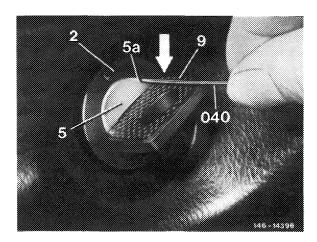
**Note:** The releasing wire is self-made from steel wire 1.25 mm thick according to adjacent drawing.
