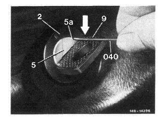
36 On both versions, insert collar into instrument panel.
