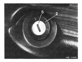
10 Introduce releasing wire (040) through bore (5a) in locking cylinder. Then push down releasing wire and unlock detent of locking cylinder by overcoming resilient resistance.
